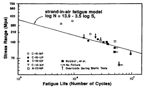
Figure 2 Fatigue of Strands in Pretensioned Girders (from [7])
