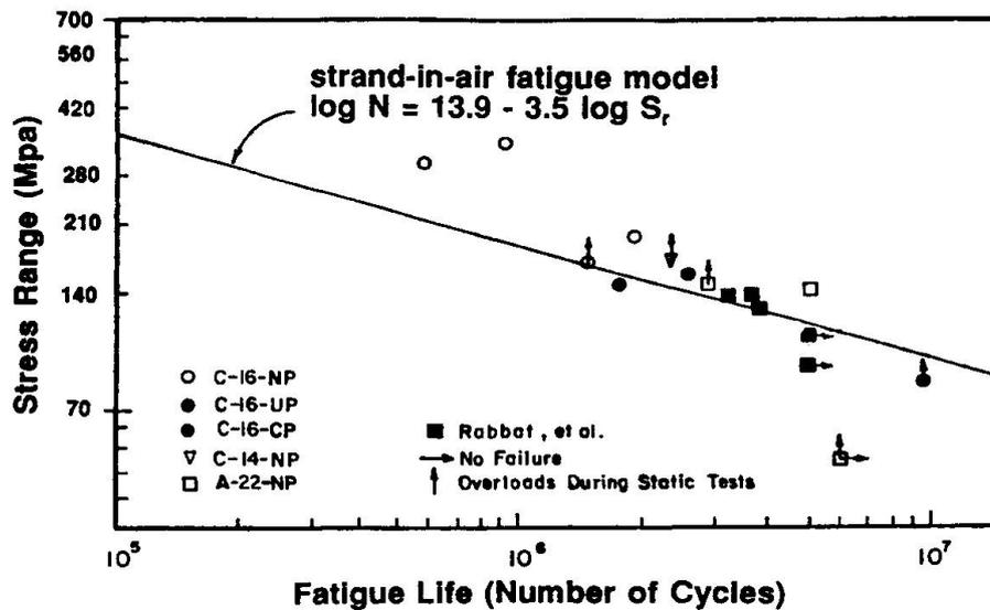
Figure 2 Fatigue of Strands in Pretensioned Girders (from [7])
