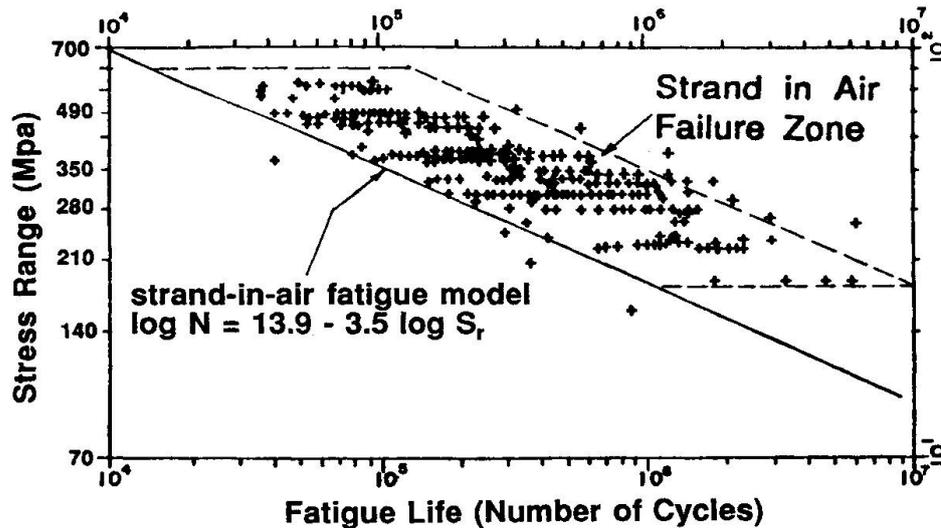
Figure 1 Strand in Air Fatigue Model (from [8])
