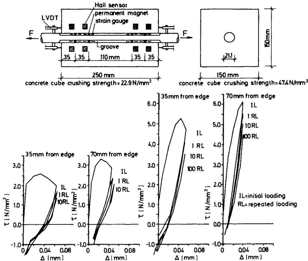
**Fig.1** Bond stress - axial displacement relations dependent on concrete strength
