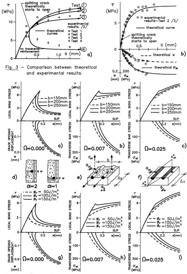
Fig.~4 — Influence of cross section width b and fracture energy  $\mathcal{G}_{F}$  on bond after splitting.
