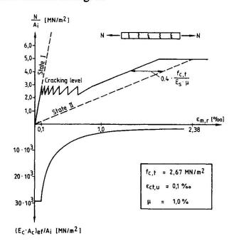
Up to the load of the first crack ( $\sigma_c = f_{c,t}$ ) the structural member remains in state I. After that a successive cracking starts. When the fully developed cracking pattern is reached, there is another ascent of the stress - strain - diagram, which is almost parallel to the plain state II, at a distance of  $0.4 \cdot f_{c,t}/E_{s} \cdot \mu$ (tension-stiffening-effect)
