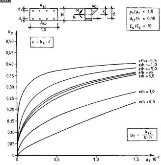
Fig. 4 Depth of compression zone under servie load
