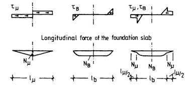
In the case of skidding friction the maximum normal force in the foundation slab results:
