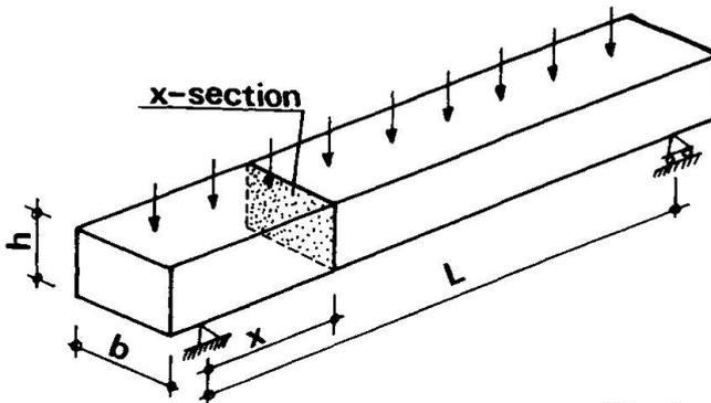
Fig. 1. Member for cracking analysis
