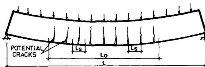
Fig. 2. Model of member with potential cracks.
