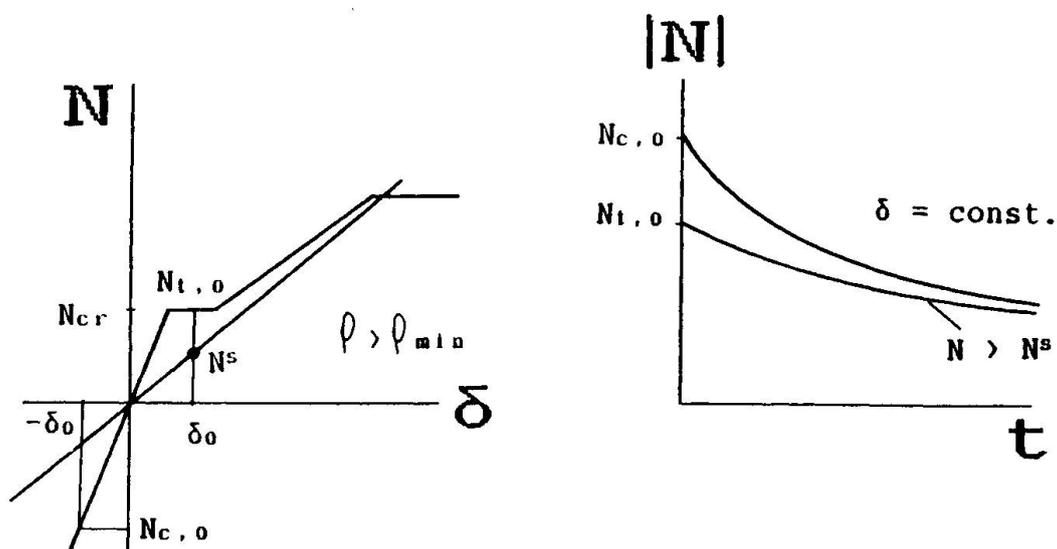
Fig. 2 a) Normal force vs. imposed deformation
