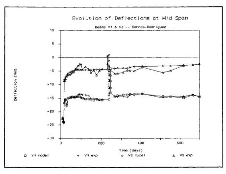
Fig. 3 Evolution of mid-span defelections
