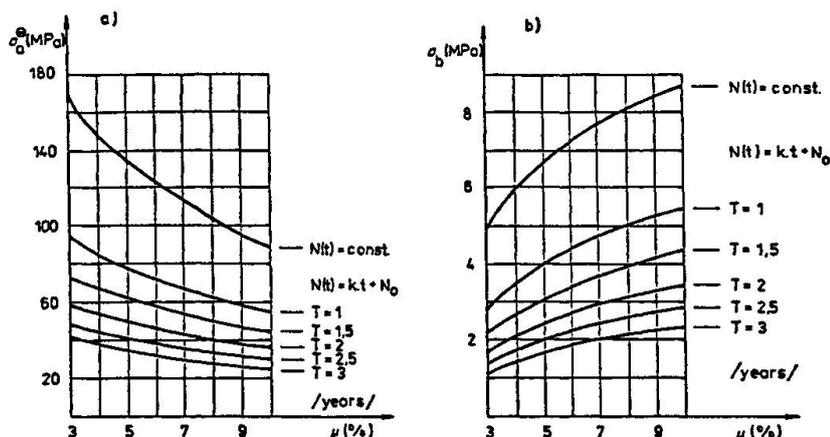
**Fig. 1** Stress in the reinforcement (a) and stress in the concrete (b) due to concrete creep at varying percentages of cross-section reinforcement, accounting for the differences in the duration of building construction time
