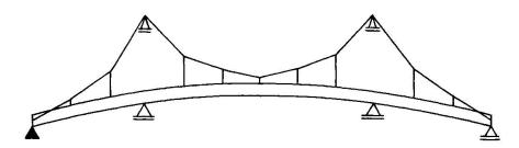
Fig. 1 - Outline of a prestressed concrete suspension bridge
