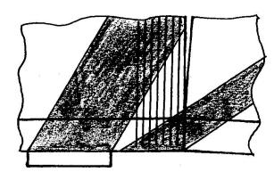
Fig. 10: Transfer of shear force from the open joint to the support, and the necessary reinforcement
