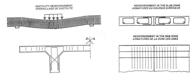
Fig. 9: Reinforcement arrangement to produce the joint ductility
