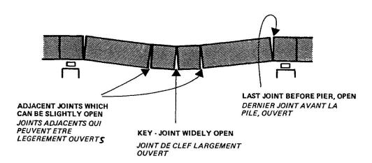
Fig. 5: Ultimate behaviour of a segmental beam
