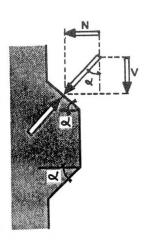
Fig. 3: Mechanical behaviour of multiple shear-keys
