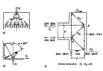
Fig. 2 Use of truss analogy to determine state of internal equilibrium
