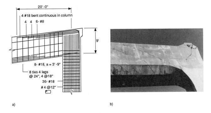
Fig. 4 Frame corner with insufficient flexural development length: (a) Reinforcement; (b) Pattern of cracks
