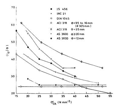
Fig. 1 ( $1d/\Phi$ ) for tension bars
