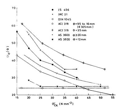
Fig. 1 ( $1d/\Phi$ ) for tension bars
