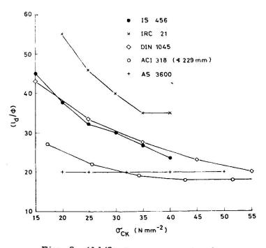
Fig. 2 ( $1d/\Phi$ ) for compression bars
