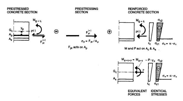
Fig. 3. Internal stresses and forces due to prestress
