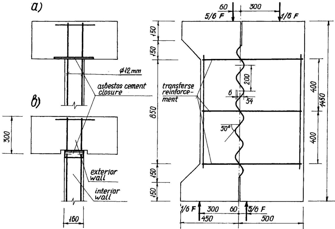
Fig. 1. Test specimens and test loading diagram of plain (a) and keyed (b) joints (dimensions in mm)
