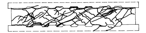
Fig. 7 Cracking at collapse
