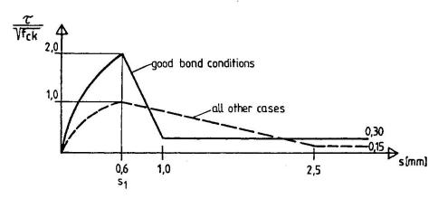
Fig. 2: Bond-Stress-Slip-Relationship of Ribbed Reinforcing Bars under Monotonic Short-Term-Loading
