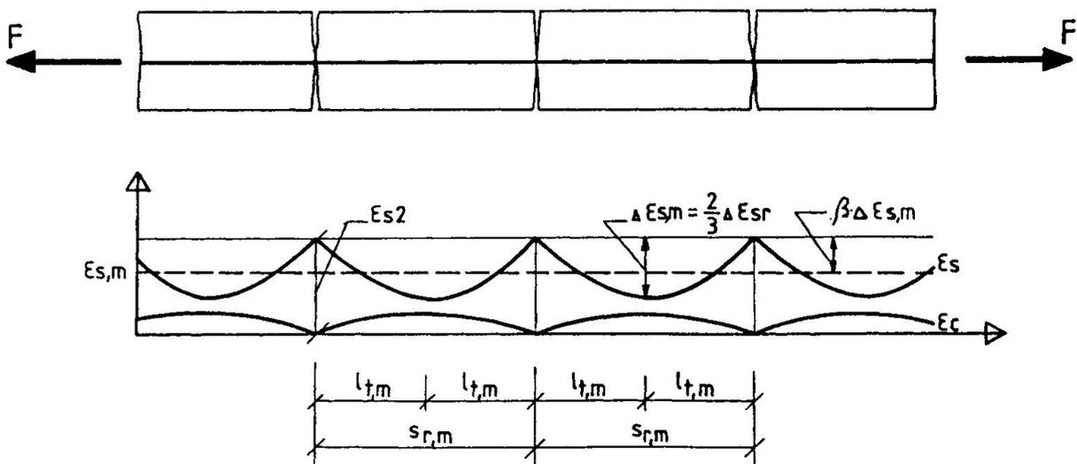
Fig. 5: Strains for average Crack Spacing  $s_{r,m}$
