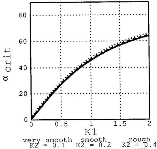
Fig. 6: crit. inclination
