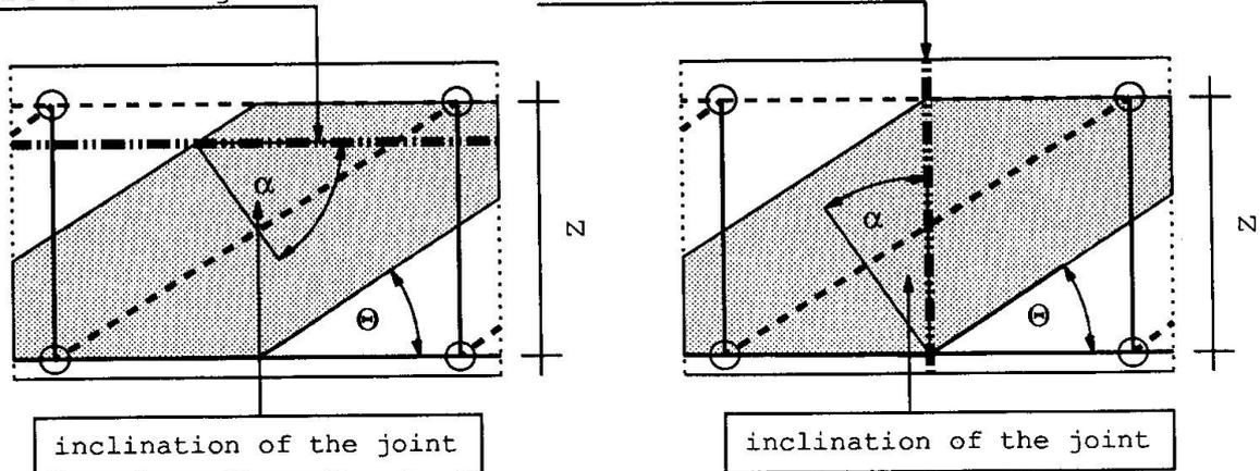
Fig. 8: strut-and-tie-model of a beam
