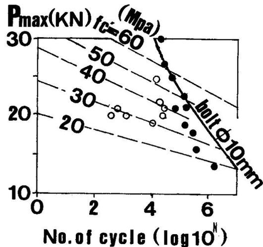
Fig.12 Fatigue Capacity
