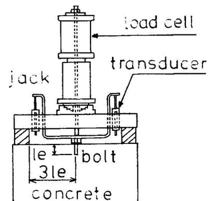
Fig.2 Test setup
