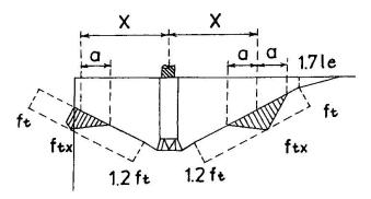
Fig. 10 Stress distribution near edge
