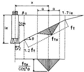
Fig.7 Proposed load carrying mechanism
