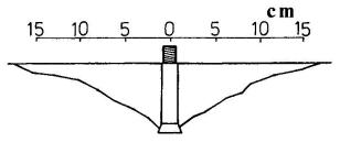
Fig.3 Ruptured cone
