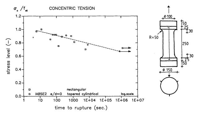
Fig. 2 Relationship between relative sustained stress level and time to failure for the concentric tensile tests
