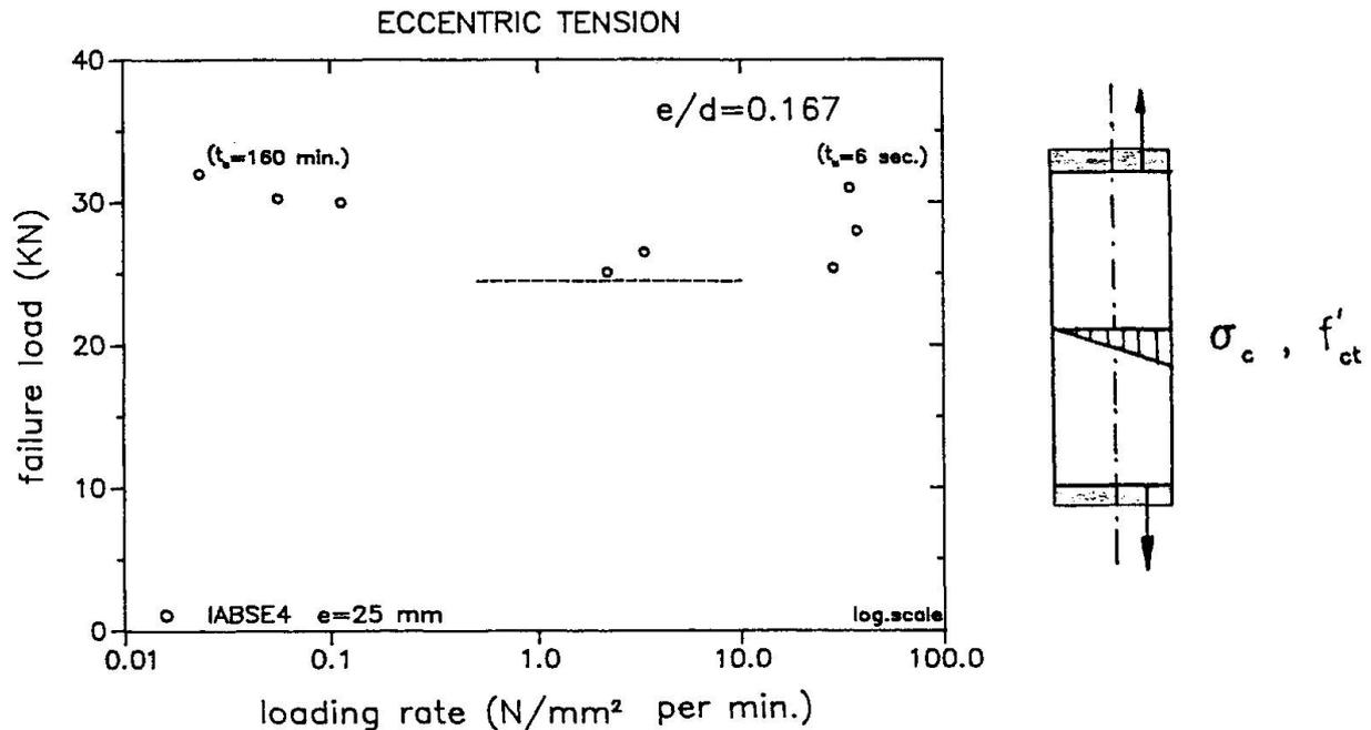
**Fig. 4** Relationship between failure tensile load and loading rate for an eccentricity of  $e/d = 0.167$
