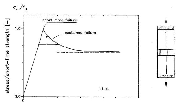
Fig. 1 Principle of sustained tensile test
