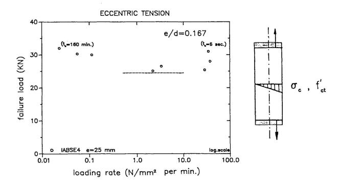
$\underline{\text{Fig. 4}}$  Relationship between failure tensile load and loading rate for an eccentricity of e/d = 0.167
