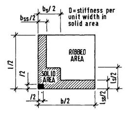
Fig. 6 Waffle slab model
