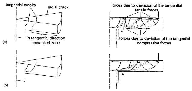
Fig. 8 Structural behaviour in the cracked state
