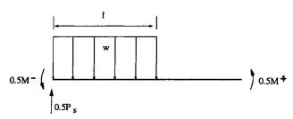
Fig. 5 Simplified Loading of Radial Half-Strip
