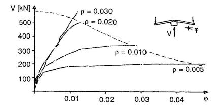
Fig. 10 Load-displacement diagrams of slabs
