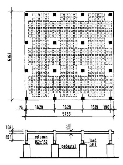
Fig. 1 Waffle slab tested by Lucio
