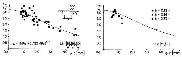
Fig. 11 Nominal punching shear strength in function of φ•d
