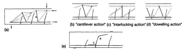
Fig. 3 Structural models after bending cracks develop with subsequent crack propagation
