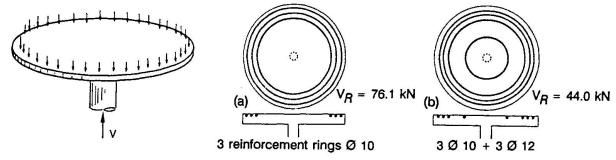
Fig. 7 Slab specimen
