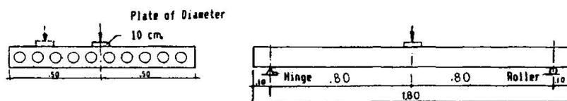
Fig. 1 Test setup for the voided slabs
