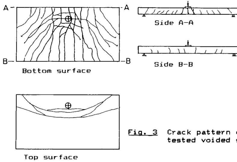
Fig. 3 Crack pattern of the tested voided slabs.
