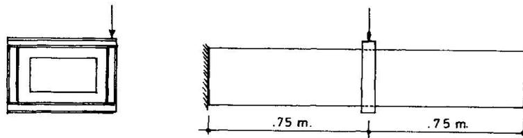
Fig. 2 Test setup for the box girders
