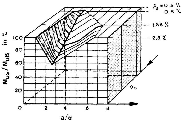
The beams were submitted to two point loads at a third of the span. Hence the shear span "a" equals 500 mm and  $a/d = 3$ . This latter value is known to be the most critical for shear strength [3]. In fig. 2 Kani's "shear failure valley" for beams without shear reinforcement is shown [3]. The diagram depicts the influence of  $a/d$  and  $\rho_s$  on the ratio of the ultimate moment corresponding to shear failure ( $M_{uS}$ ) to the ultimate moment for bending failure ( $M_{uB}$ ).
