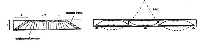
Fig. 6 Model for simply-supported beams.
