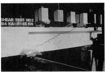
Fig. 3 RC T-beams under six-point loading. Design details and mode of failure [6].
