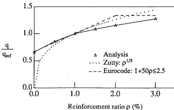
Fig.5. Influence of reinforcement ratio  $\rho$
