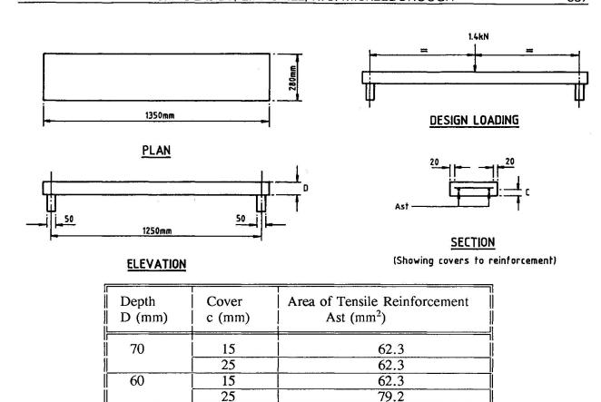
Fig. 2 Plank Design Details
