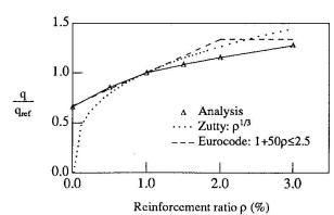
Fig. 5. Influence of reinforcement ratio  $\rho$  (1/d=9, d/l<sub>ch</sub>=3.0, for  $q_{ref}$ :  $\rho$  = 1%)
