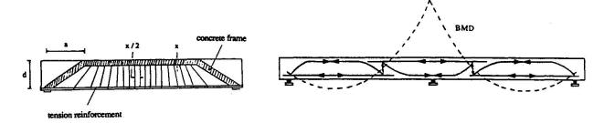
Fig. 6 Model for simply-supported beams.
