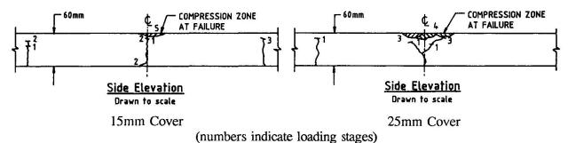
Fig. 5 Cracking Patterns - Impact Loading 60mm Thick Planks
