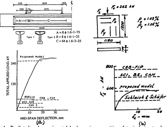
Fig. 1 Predicted and experimental load-carrying capacities of typical structural concrete members tested by (a) Kotsovos & Lefas [11] and (b) Maier & Thurlimann [12].
