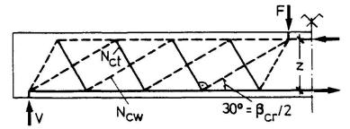
Fig.4: Truss model for members without transverse reinforcement
