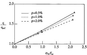
Fig. 6. Influence of axial compressive stress (1/d=9, d/l<sub>ch</sub>=3.0, for  $q_{ref}$ :  $\sigma_N = 0$ )
