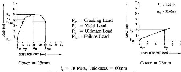
Fig. 3 Load/Displacement Plots - Static Loading
