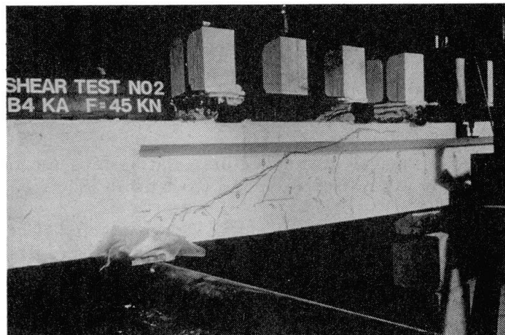
Fig. 3 RC T-beams under six-point loading. Design details and mode of failure [6].
