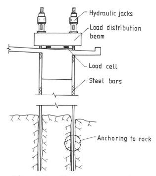
Fig. 5 Loading arrangement
