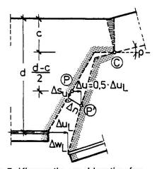
Fig.5: Kinematic consideration for crack width
