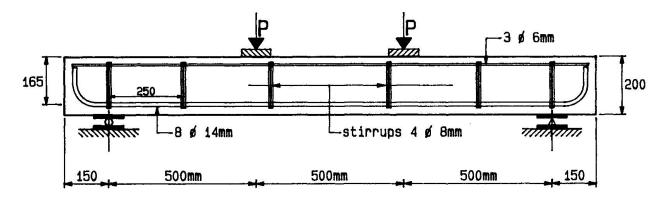
Fig. 1 Dimensions and reinforcement of beams R/1.86/0.20 and L/1.86/0.20
