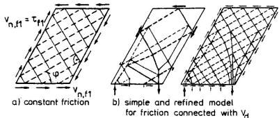
Fig.3: Stress fields between cracks
