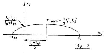
From the shear stress-diagram the shear force  $V_{\rm C}$  can be calculated [2][3].  $V_{\rm C}$  as well as  $N_{\rm C}$  are parameter functions of the deformation  $\varepsilon_{\mathrm{cu}}$  of the concrete on  $\sigma_{\rm c}$  the upper side.
