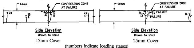
Fig. 4 Cracking Patterns - Static Loading 60mm Thick Planks
