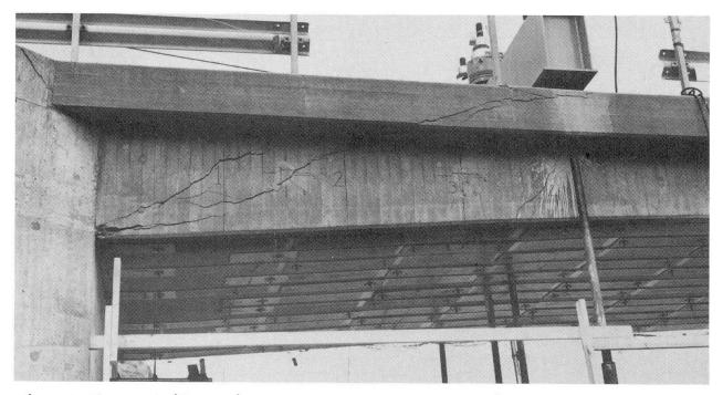
Fig. 6 Shear failure in the non-prestressed bridge
