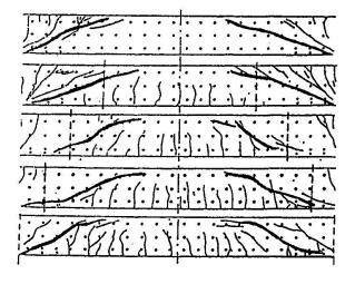
Fig. 1 Five different moment lines (5 different moment parameters) and the respective crack patterns of the beams. All beams have the slenderness parameter  $l_0/d = 4.5$  and d = 150 mm
