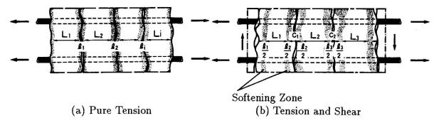
Fig.2 Reinforcement Induced Strain Fields of Concrete
