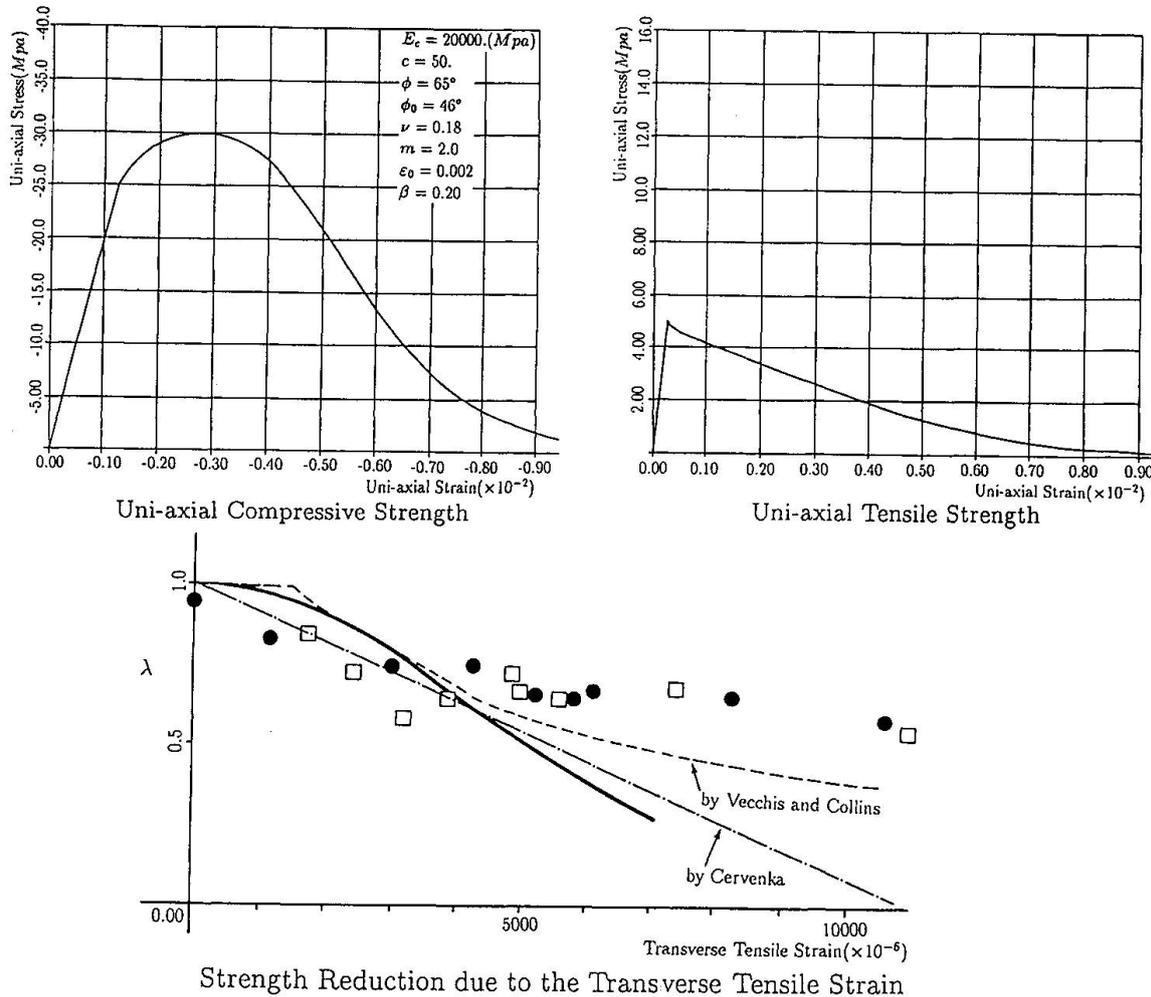
Fig.9 Strength Reduction Calculated
