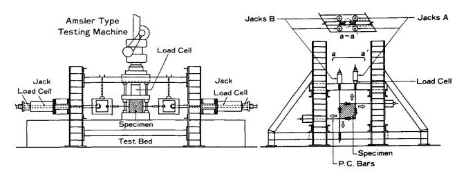
Fig. 7 Shirai's Testing Method
