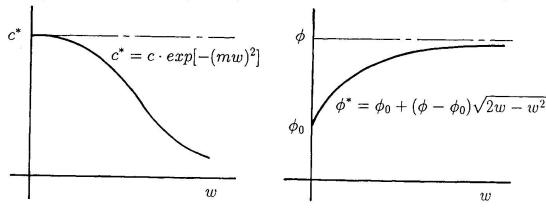
Fig.3 Possible Relations of  $c^* - w$  and  $\phi^* - w$
