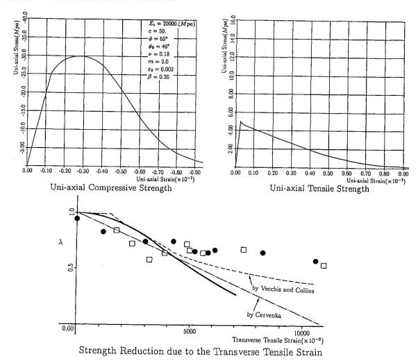
Fig. 9 Strength Reduction Calculated
