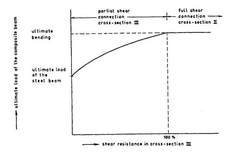
Figure 9: Qualitative relation between the ultimate load and the longitudinal shear resistance
