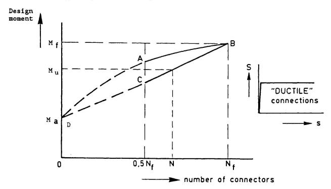
Figure 16: Relationship between design moment and number of shear connectors for ductile connectors
