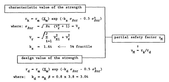
Figure 24: Characteristic value of the strength
