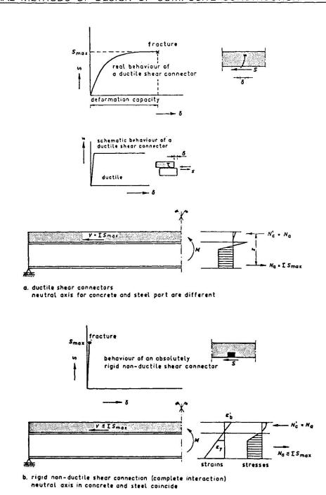
Figure 12: The influence of the deformation capacity of shear connectors on the strain and the stress distribution in case of a partial shear connection
