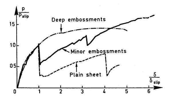
Figure 34: Load-deformation curves for composite slabs
