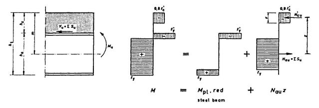
Figure 15: Stress distribution if the shear connection is partial
