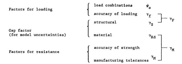
The format of the formula for the design resistance R should be consistent with Eurocode 2 and Eurocode 3. However in Eurocode 2 the partial safety factor  $\gamma_{\rm M}$  for concrete and reinforcing steel are applied to properties of the materials while in Eurocode 3 the factor  $\gamma_{\rm M}$  is applied to the resistance of cross-sections or members.
