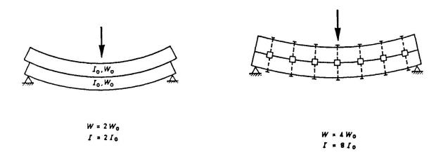
Figure 6: Illustration of composite action
