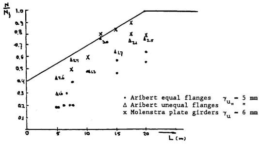
$\begin{array}{c} \underline{\text{PROPOSED RELATION FOR EUROCODE 4}} \\ \text{Plate girders with unequal flanges} \\ \underline{\text{Ab}} \\ \underline{\text{Au}} \end{array}$
