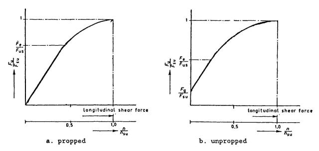
Figure 14: Relation between the load and the longitudinal shear force i.e. the degree of shear connection, when rigid non-ductile shear connectors are applied.
