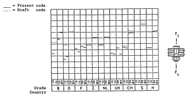
Figure 20: Non-dimensional comparison for the allowable tensile-force in bolts
