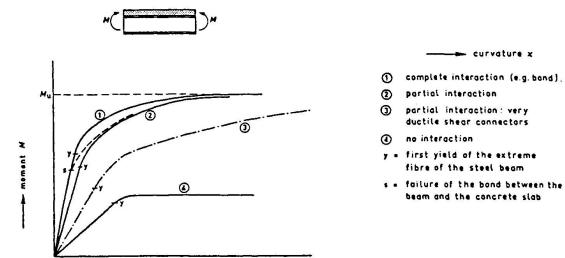
Figure 11: Influence of slip on a M-κ diagram
