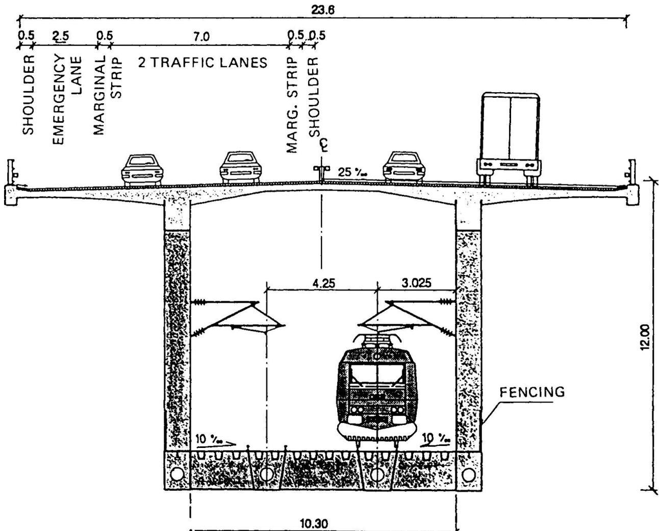
Fig.24 Cross section
