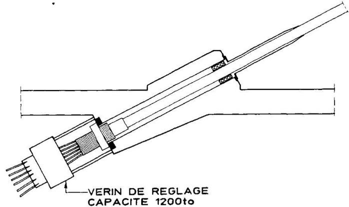
Fig.41 Tensioning jack
