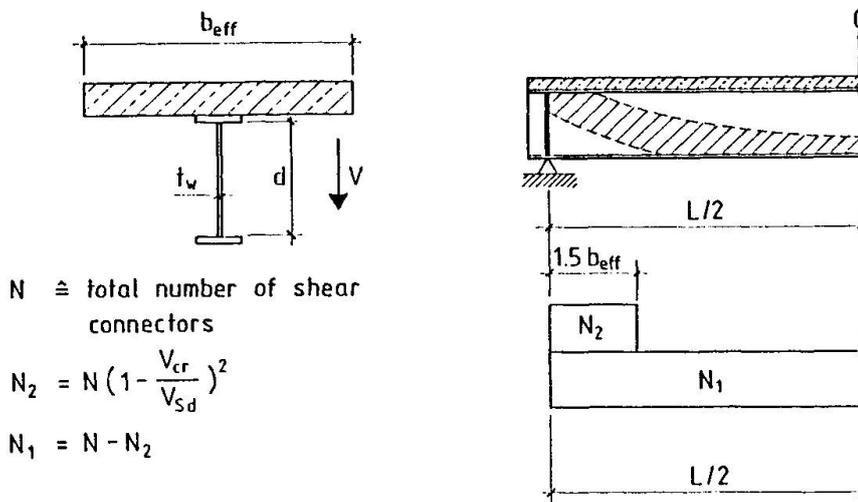
Fig. 20 Distribution of shear connectors, when  $V_{sd} > V_{cr}$
