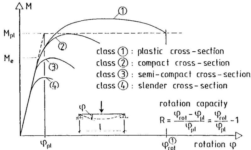
Fig. 5 Rotation capacity and cross section classes
