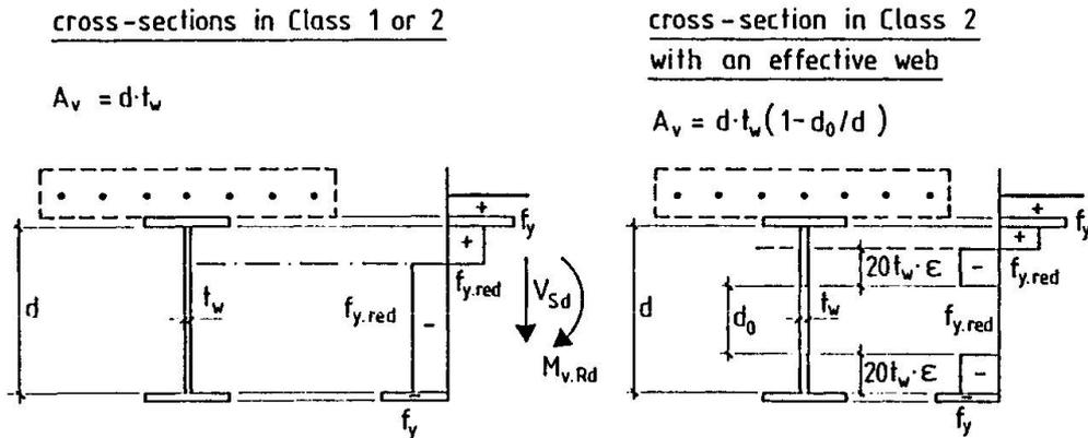
Fig. 21 Reduced yield strength for the steel web
