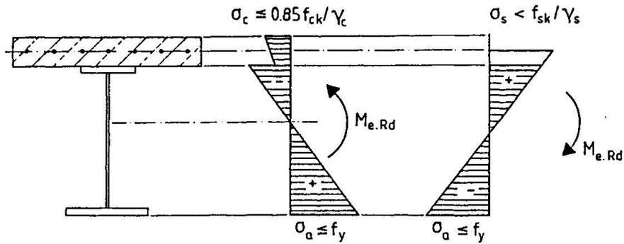
Fig. 14 Elastic stress distributions for sections in Class 3
