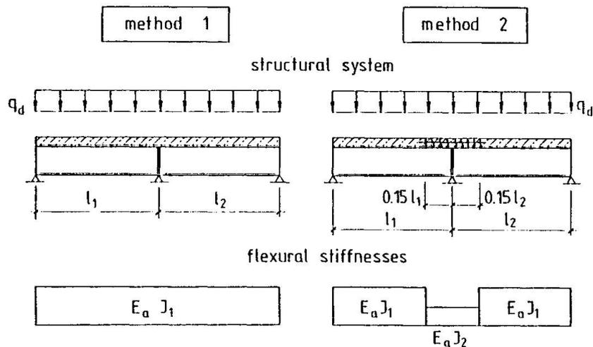
**Fig. 7** Calculation of internal moments by elastic global analysis
