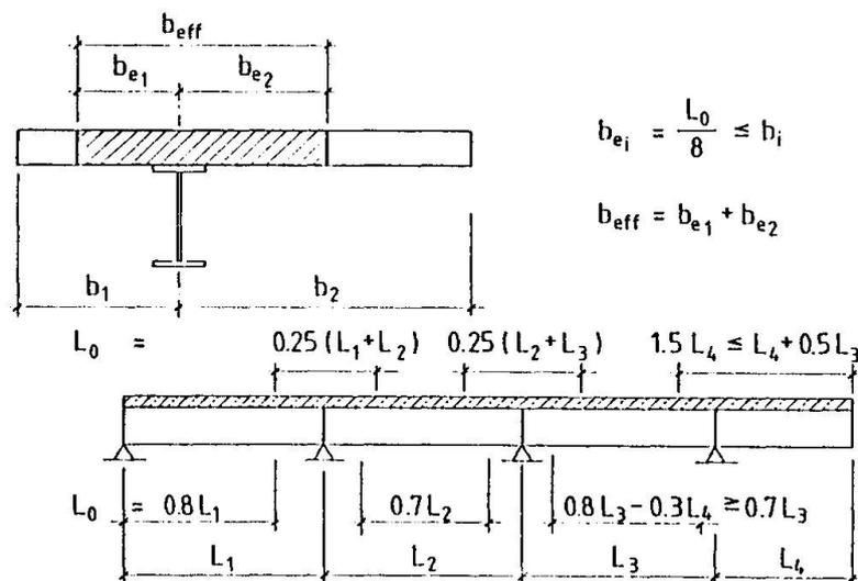
Fig. 9 Effective width of concrete flange
