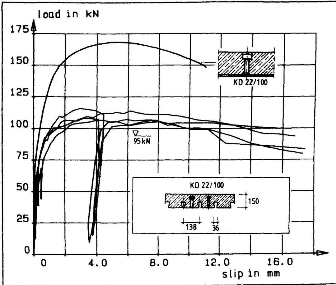
Fig. 16 Load - slip curves of stud shear connectors
