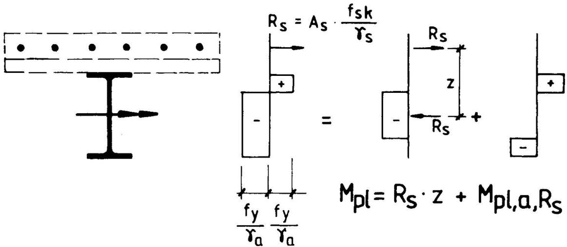
Fig. 10 Hogging bending moment
