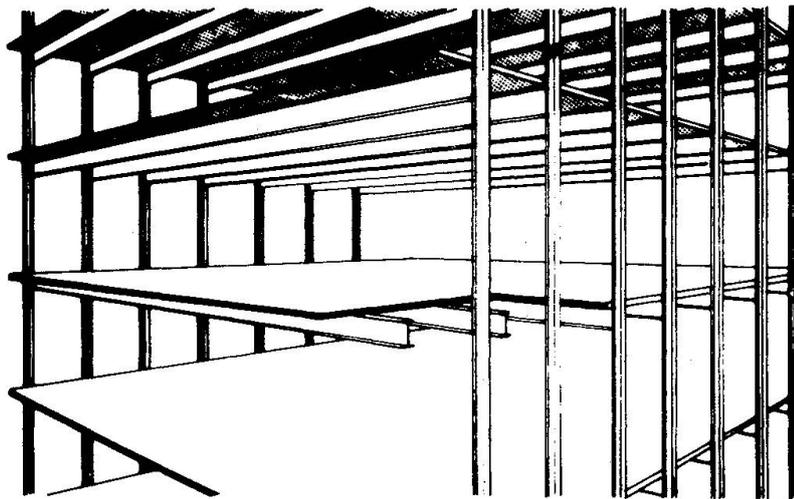
Fig. 1 Composite floor constructions for office buildings
