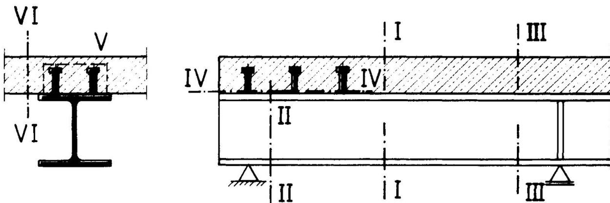
Fig. 5 Critical sections which have to be checked
