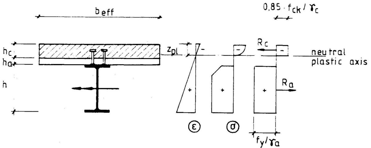
Fig. 6 Strain and stress distribution (sagging bending moment)
