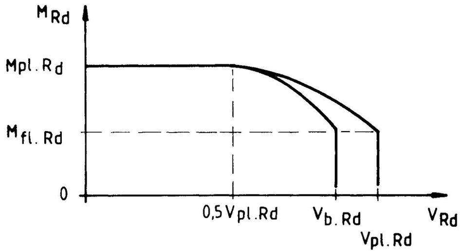
Fig. 11 Interaction for bending and vertical shear
