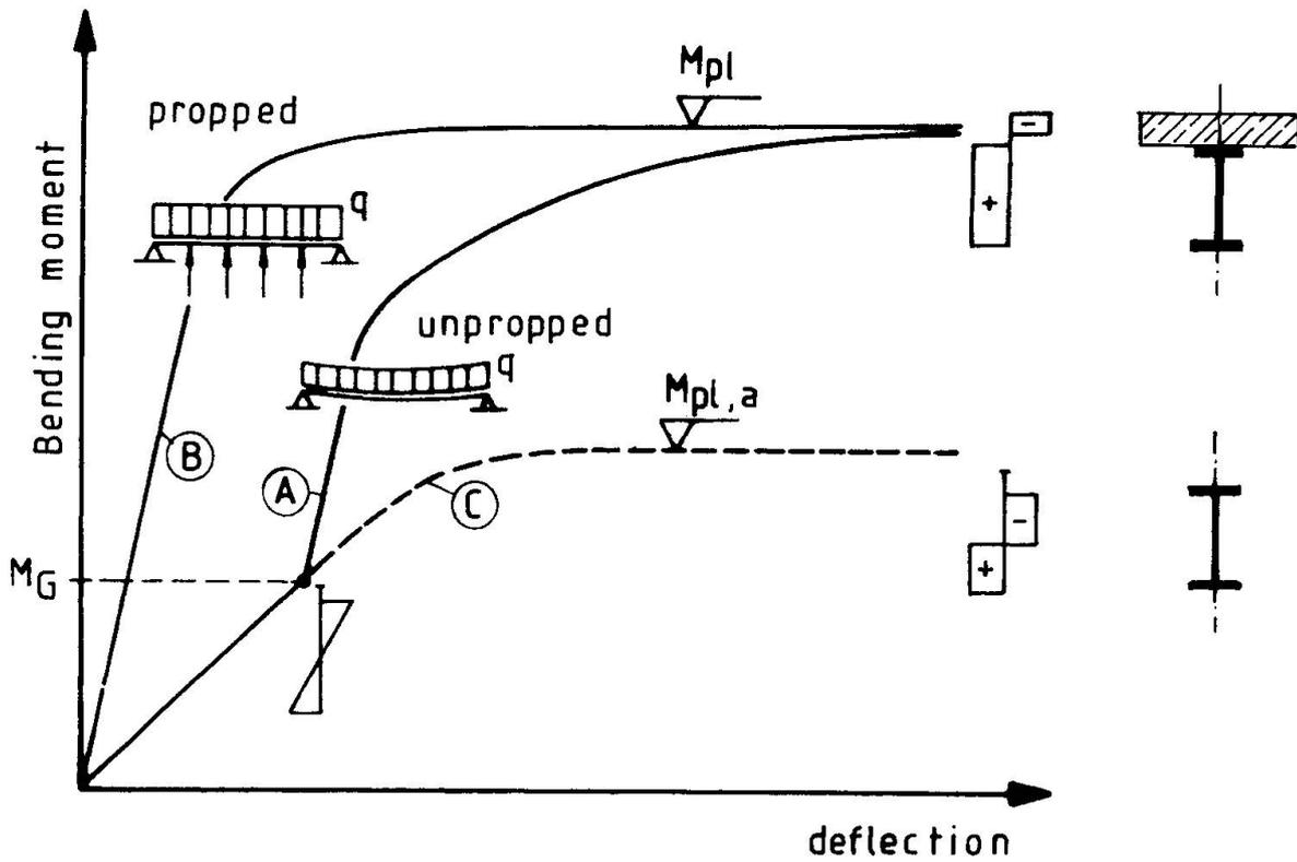
Fig. 4 Effects of propped and unpropped construction
