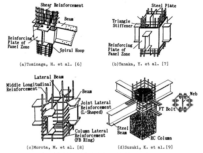
Fig.4 Jointing Methods between RC Column and S Beams in Previous Researches
