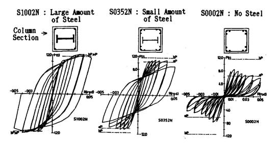
Fig. 3 Test Results on Beam-Column Joints from Type 2 (RC Column) to Type 1 (SRC Column) (Wakabayashi, M. et al. [5]
