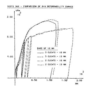
Figure 2 - Influence of the percentage of reinforcement in the concrete slab (connections with IPE 360 beams no upper flange cleat)
