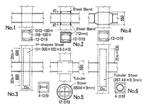
Fig. 3 Joint Details of Specimens
