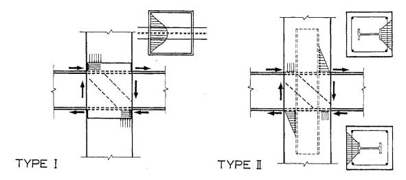
Fig. 7 Stress Transfer Mechanism
