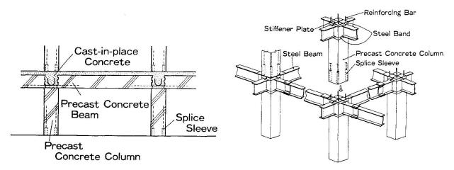
Fig. 1 Precast Concrete Frame System
