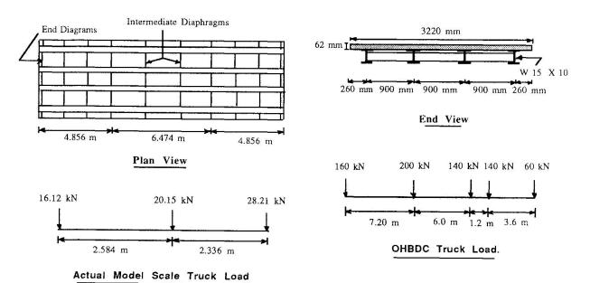
Figure 1. Details of Bridge Model and Loading.
