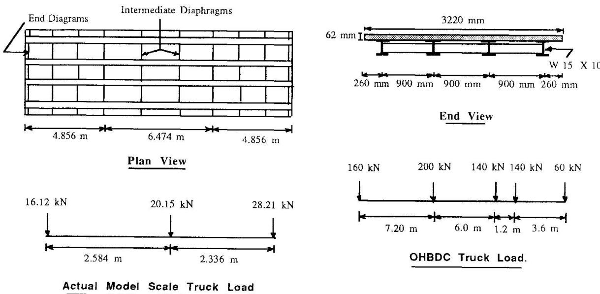
Figure 1. Details of Bridge Model and Loading.
