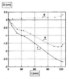
Fig. 8 Vertical diplacements of the top of the lower columns
