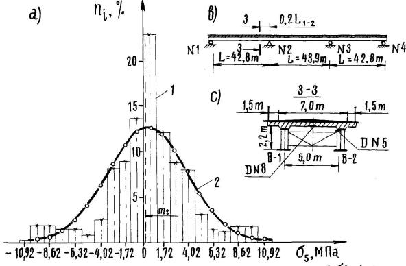
Fig. 2. The diagram of stress probability density (6; ) in the upper flange of the bridge girder B - 2 in the span L<sub>4-2</sub> (section 3-3): 1 - in according to the experimental data; 2 - the theoretical destribution normal law.
