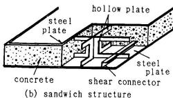
Figure 1 Composite structures
