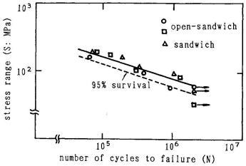
Figure 5 S-N relationship of steel plates
