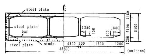
Figure 9 Cross section of the tunnel element
