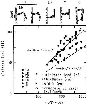
Figure 2 Load-carrying capacity of shear connectors
