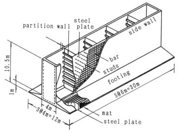
Figure 7 Details of the caisson
