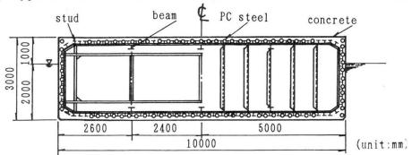
Figure 6 Cross section of the floating body
