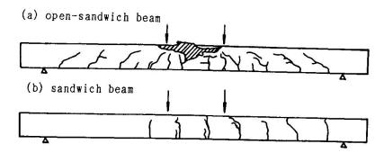
Figure 3 Crack formation
