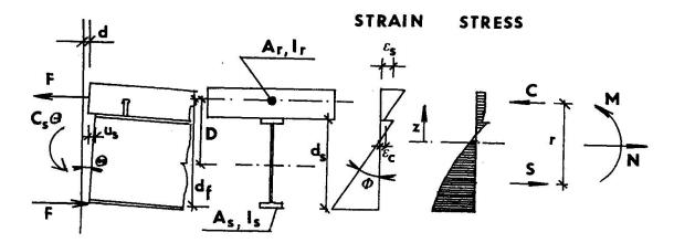
Fig. 1 The Composite Beam Element Model
