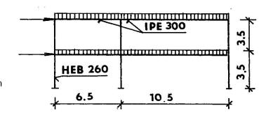
Fig. 3 Frame Configuration
