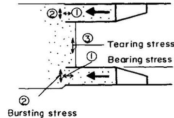
Fig. 6 Local stress at the connected part
