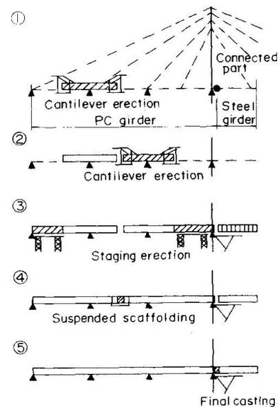
Fig. 7 Constructing sequence of the connected part
