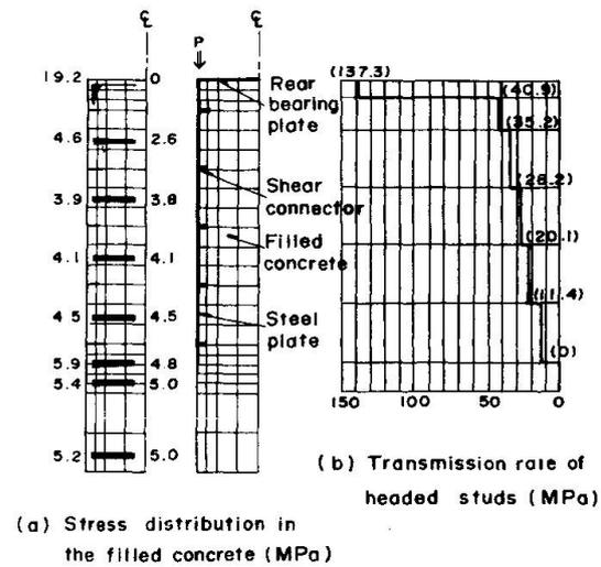
Fig. 5 Transmission mechanism of the filled concrete
