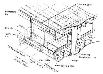
Fig. 2 Perspective of connected part
