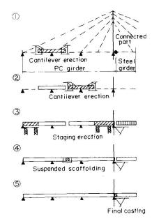
Fig. 7 Constructing sequence of the connected part
