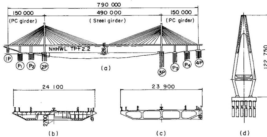
Fig. 1 Ikuchi Bridge : (a) Side view (b) Steel girder section,
