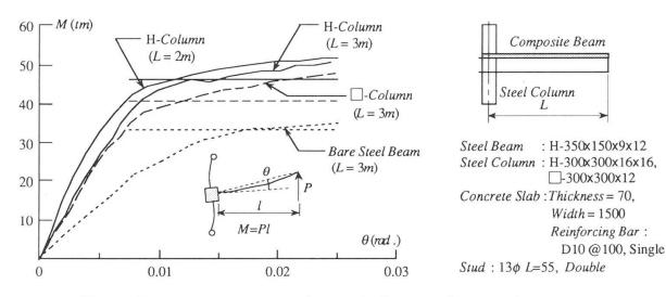
Fig. 11 Moment-rotation curves of composite beams and test specimens
