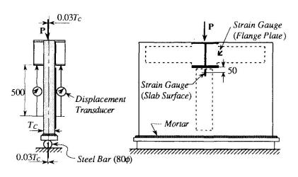
Fig. 7 Test setup
