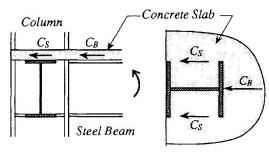
Fig. 2 Transmission of compressive force in the concrete slab
