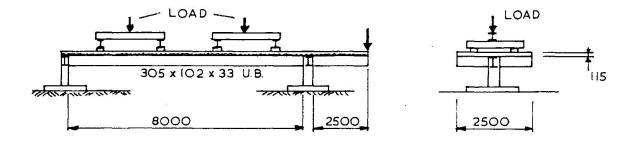
Fig. 1 Test arrangement
