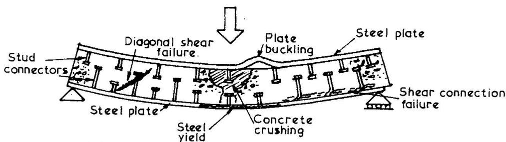
Fig. 1 Double skin composite construction
