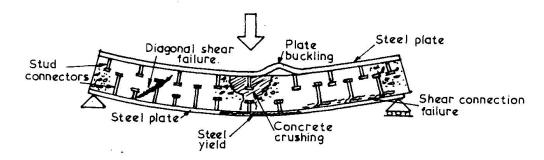
Fig. 1 Double skin composite construction
