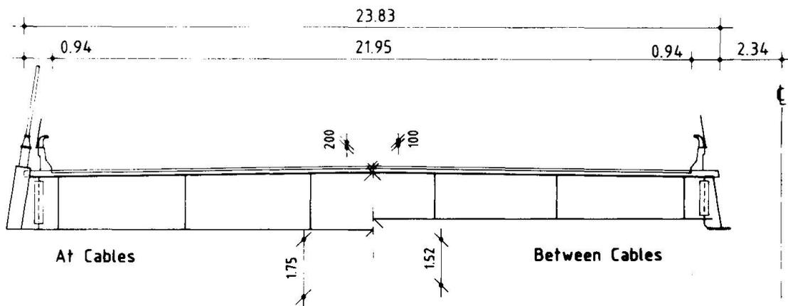
Fig. 2 Individual Beam Cross-Section
