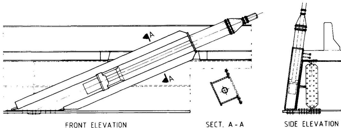
**Fig.4** Stay Cable Anchorage at Beam
