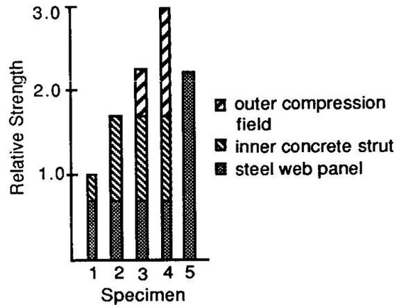
Fig. 6 Comparison of Joint Strengths
