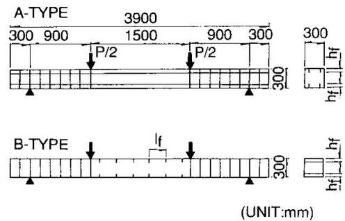
Fig. 1 Flexure test models and loading configurations
