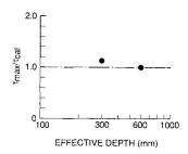
Fig. 9 Experimental/calculated shear strength
