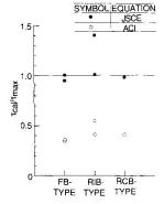
Fig. 6 Experimental/calculated shear strength
