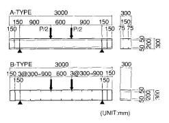
Fig. 4 Shear test models and loading configurations
