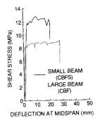
Fig. 8 Shear stress - deflection curves
