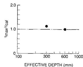
Fig. 9 Experimental/calculated shear strength
