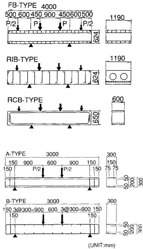
Fig. 4 Shear test models and loading configurations
