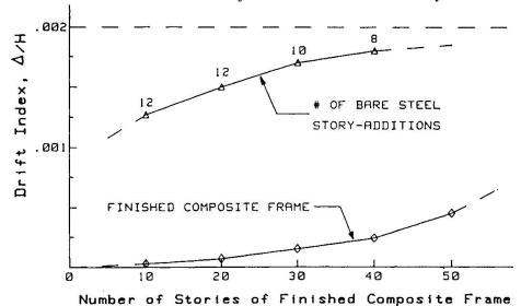
Figure 3 Drift vs. Number of Stories of Finished Composite Frame
