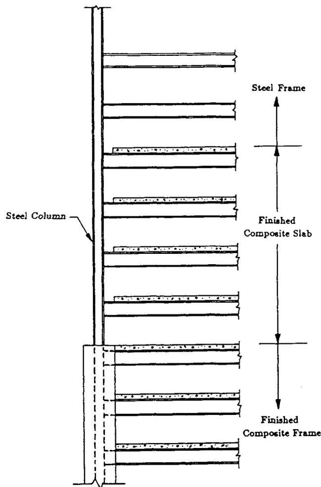
Figure 1 Construction Sequence of a Composite Frame
