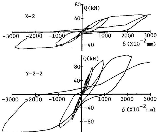
Fig.3 Load(Q)-displacement(δ) curves under repeated loading
