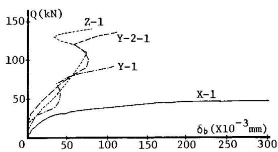
Fig.4 Load(Q)-displacement of base plate(δ\_b) curves
