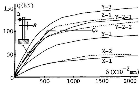
Fig.2 Load(Q)-displacement(δ) curves under monotonic loading
