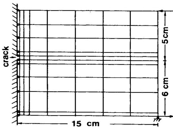
Fig. 3 Finite elements net.
