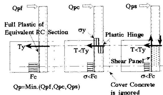
Fig.2 Collapse Mechanisms
